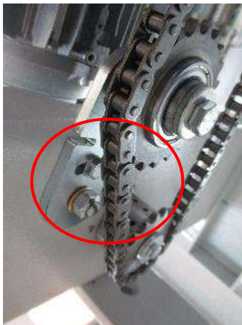
DETAIL SCREW LOCKING IN SLOTS - BOTTOM VIEW
