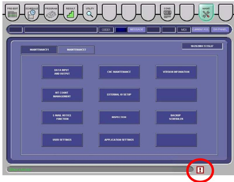
If there is any overdue inspection item, it is indicated by an icon at the lower right of the display. The icon disappears when all inspection items are finished to leave no overdue inspection items.
