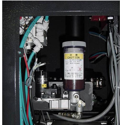
A grease cartridge recommended for use with the automatic grease lubricator contains 400 cm<sup>3</sup> {13.5 fl.oz.} of grease and can accommodate about 167 grease lubrication times.
