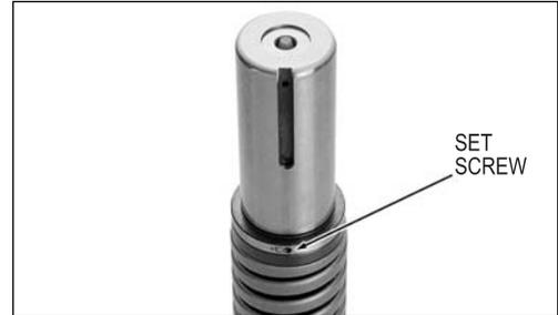
When the punch guide is not fastened with the set screw, use the QS pliers to disassemble the punch guide. How to use the QS pliers is described below.
