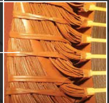
Anti-Bacterial Coating on Windings
