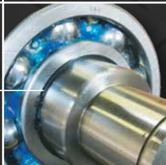
Snap Rings Holding Bearing in Place
