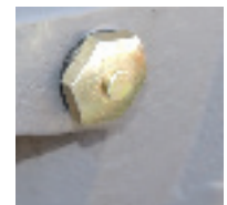
Grease pressure reliefs act to battle overgreasing
